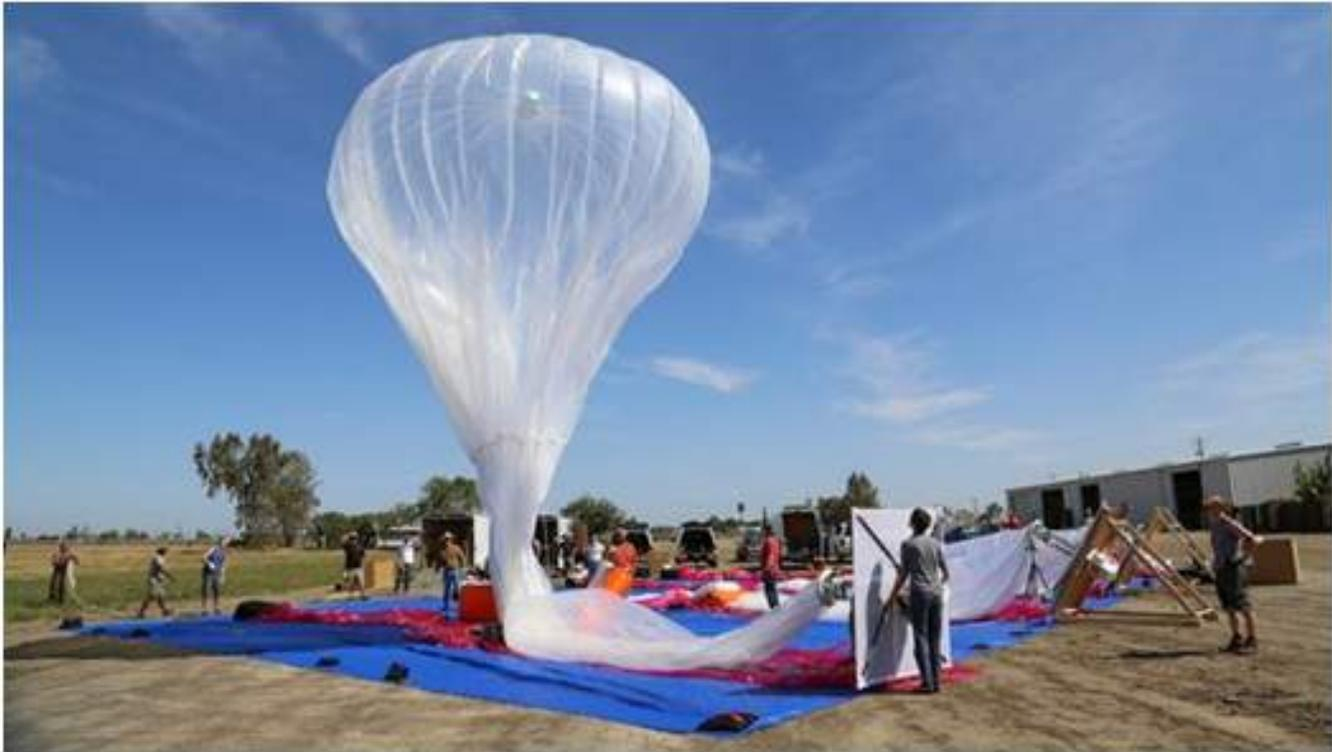
The balloon envelopes used in the project are made by Raven Aerostar, and are composed of polyethylene plastic about 0.076 mm (0.0030 in) thick. The balloons are super pressure balloons filled with helium, standing 15 m (49 ft) across and 12 m (39 ft) tall when fully inflated. They carry a custom air pump system dubbed the "Croce" that pumps in or releases air to ballast the balloon and control its elevation.
